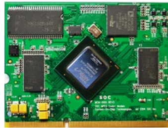
Fig. 2 The SOC MCM-1000A Modules
