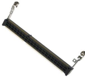
Fig. 8: A photo of the standard 204 pin DDR3 SODIMM connector
