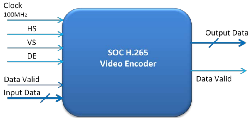
Fig. 4 The inputs and outputs of the H.265 video encoder IP Core
